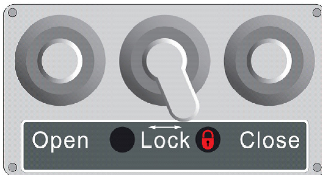
Figure 0.3 — Example of door lock providing visual and tactile indication of status
